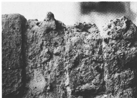
Figure 1. Surface of a 16th century Venetian brick eroded by rain water run-off. A highly-vitrified nodule resists deterioration better than the less vitrified matrix.
