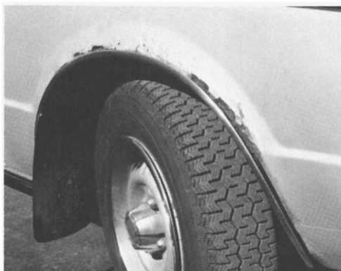
Auto body corrosion adjacent to stainless steel trim occurs in environments where de-icing salts are used. The effects of acid deposition combined with road salts produces a synergistic effect on the degradation of automobiles. (Photo by Robert Baboian.)
